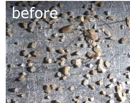
Natural “siderite” in experiment with CO 2 + 4% O 2
