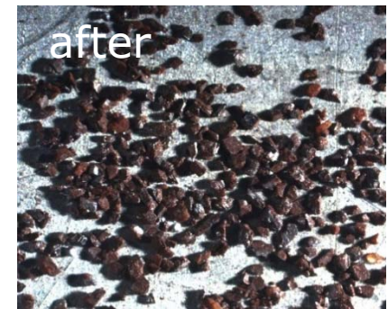
Natural “siderite” in experiment with CO 2 + 4% O 2
