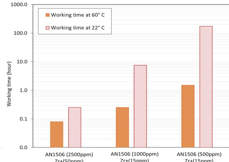
For higher concentrations of AN1506 and AN907PG, working time was significantly reduced with increase in temperature.
